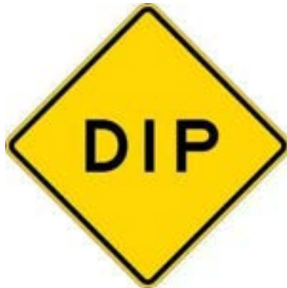
Sample of dip (sag curve) advanced warning sign (W8-2) from the MUTCD
